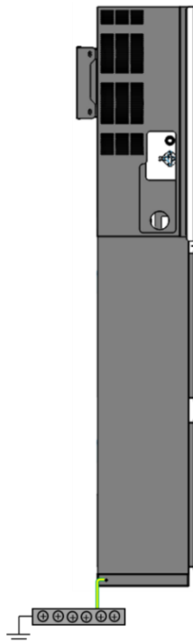
Figure 5-6: Earth Connection between Ground and Cabinet
