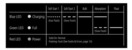
CHARGING LED: blue LED illuminates and flashes during charging process. FULLY CHARGED LED: green LED illuminates (solid) when fully charged.
