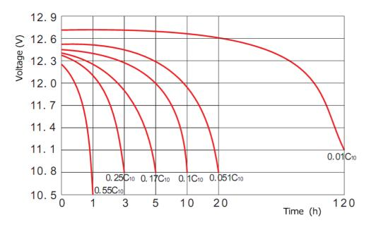
Table 2-1 NLC Series Battery End Voltage at Different Discharge Rate (25℃)
