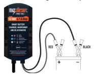
If the Battery is out of the vehicle: Connect the Red/Orange (+) Crocodile clip or ring terminal to the positive (+) battery terminal. Connect the Black (-) Crocodile clip or ring terminal to the negative (-) battery terminal.
