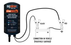
If **Positively Earthed** – FIRST Connect the Black (-) Crocodile clip or ring terminal lead to the negative (-) battery terminal and then connect the Red/Orange (+) Crocodile clip or ring terminal lead to the vehicle's chassis or positive (+) battery terminal. DO NOT connect the Red/Orange (+) lead to the carburettor or fuel lines.
