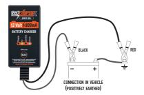
If **Positively Earthed** – FIRST Connect the Black (-) Crocodile clip or ring terminal lead to the negative (-) battery terminal and then connect the Red/Orange (+) Crocodile clip or ring terminal lead to the vehicle's chassis or positive (+) battery terminal. DO NOT connect the Red /Orange (+) lead to the carburettor or fuel lines.
